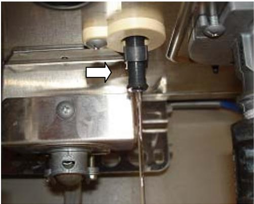
18. Close the cold water main valve and clean the water filter. Place the filter back into the unit
